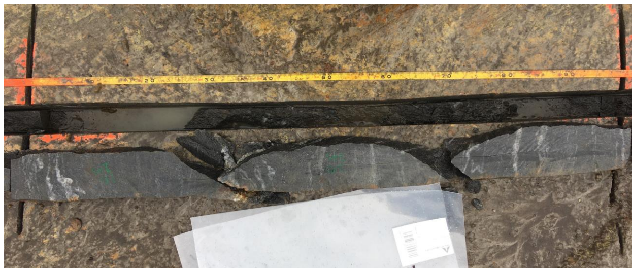
Figure 9-3: Channel sample Y092084 (10.9 g/t Au over 1,0 m) Metasediments (meta-greywacke) with 3% pyrrhotite, 3% arsenopyrite and 5% millimetric quartz-feldspar veinlets.
