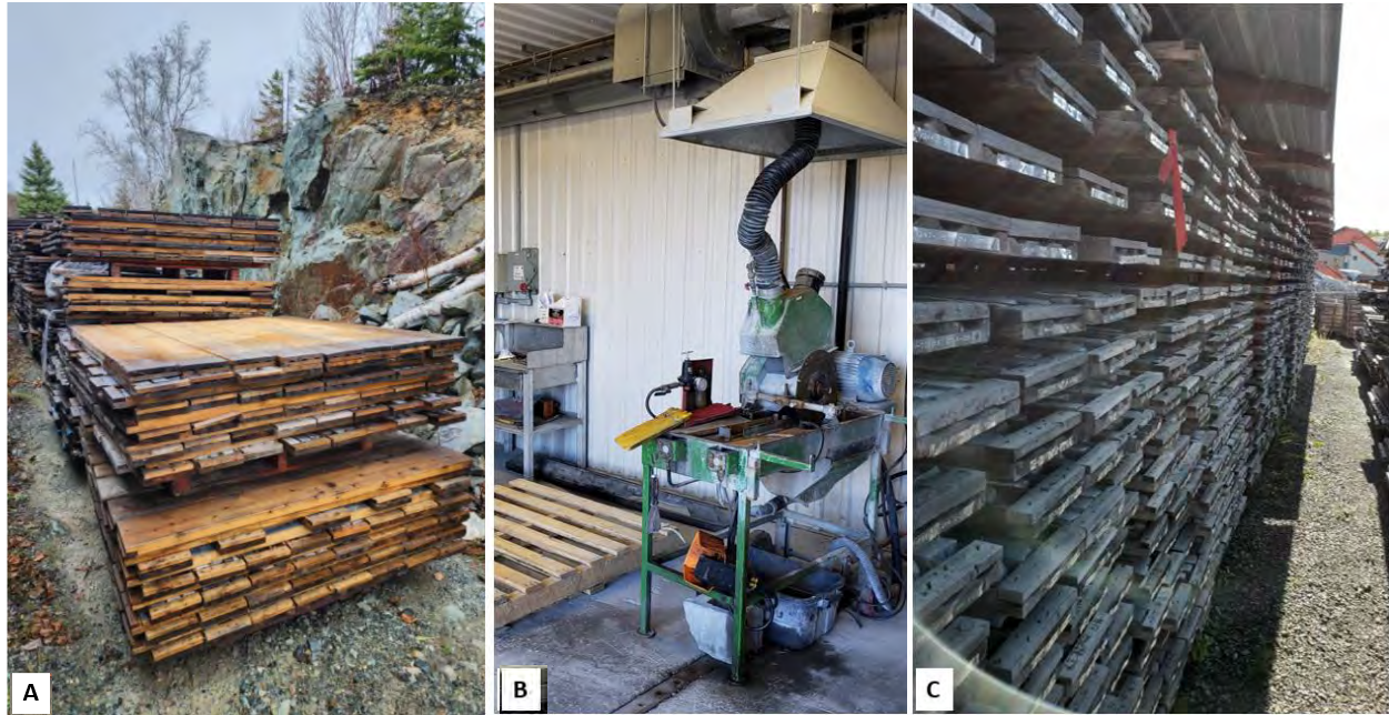
Figure 12-1: Storage and sampling procedures reviewed during some visits at the Rouyn-Noranda facilities A) Palletted drill core boxes; B) Core saw used to sample the core; C) Roofed drill core storage
